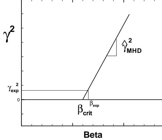
FIG. 1: The variation of growth rate with free energy, as parameterized by  $\hat{\gamma}_{MHD}$ , is nearly as important as the location of the marginal point in interpreting experimental results.
