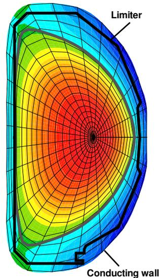
FIG. 6: In axisymmetric equilibrium, the plasma region contains a hot region where the field lines are closed and a cold, halo plasma where the field lines strike the wall. Dirichlet boundary conditions are applied at the vacuum vessel.
