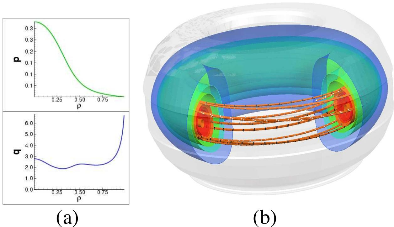
FIG. 8: (a) Equilibrium reconstruction of DIII-D discharge 87009 at  $1675\text{msec}$  shows a reverse shear profile and peaked pressure profile. (b) The three dimensional plots of the simulation include temperature isosurfaces, magnetic fieldlines colored according to temperature, and the heat flux on the limiter.
