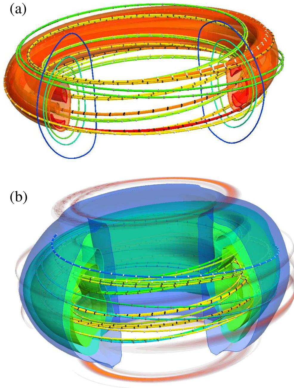
FIG. 9: In axisymmetric equilibrium, the plasma region contains a hot region where the field lines are closed and a cold, halo plasma where the field lines strike the wall. Dirichlet boundary conditions are applied at the vacuum vessel.
