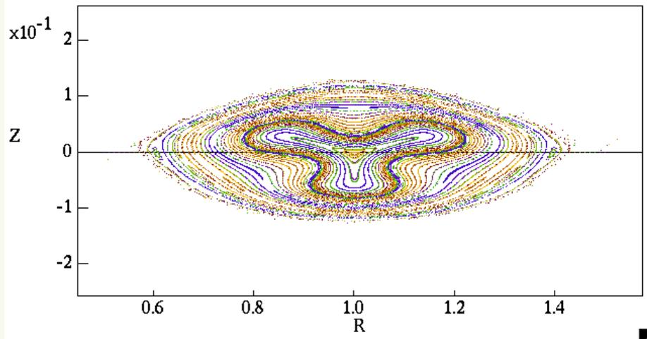
Figure 5: Poincaré plot for the helically symmetric case at  $t=1.72\text{ms}$ ,  $\zeta = 0$ .
