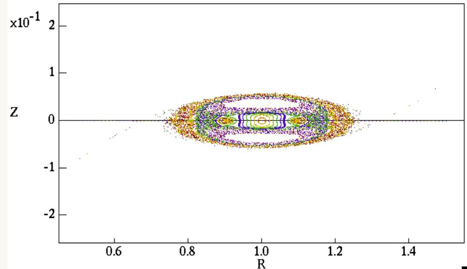
Figure 16: Poincare plot for the spoiled-symmetry case at  $t=2.55\text{ms}$ ,  $\zeta = 0$ .
