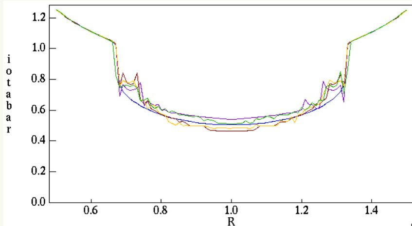
Figure 18: Rotational transform profile at various times,  $\zeta = 0$ .
