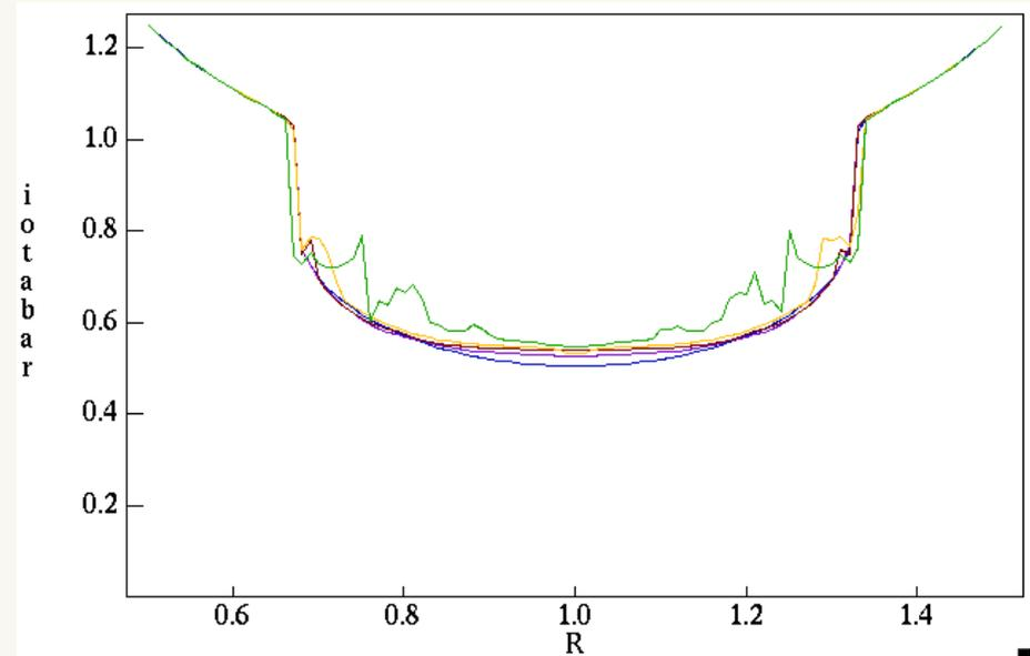
Figure 13: Rotational transform profile at various times,  $\zeta = 0$ .
