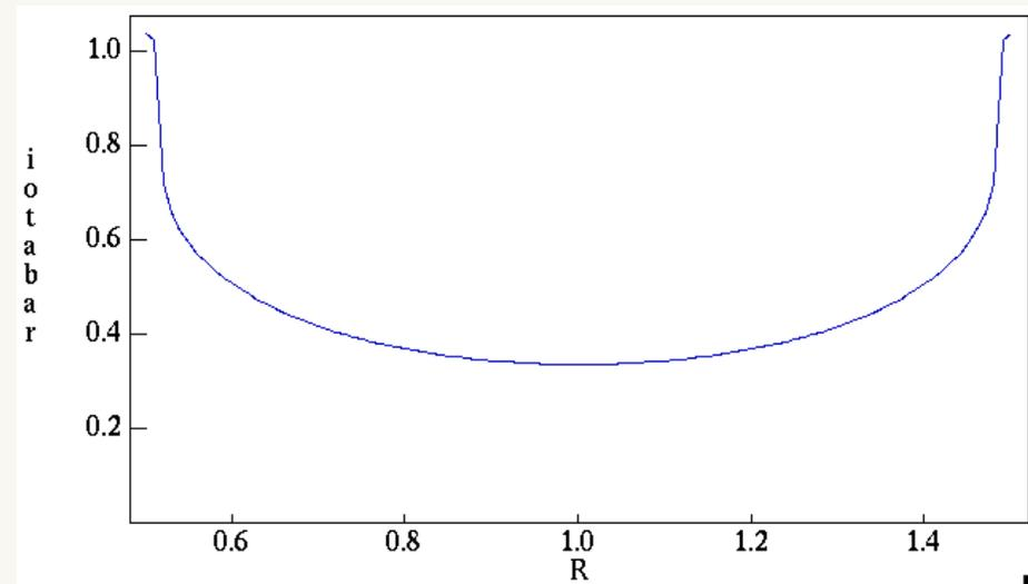
Figure 2: Rotational transform profile at  $t=0$ ,  $\zeta = 0$ .
