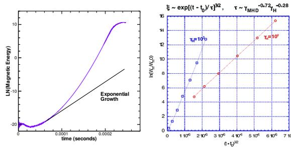
Figure 1: In 1a (left), the mode clearly grows faster than exponential. In 1b (right), both heating rates give good fits to the scaling of Eq. (1) as shown by the straight lines.
