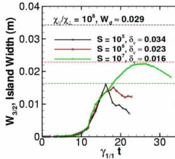
Figure 4: Simulations of DIII-D discharge 86144 show sensitivity to the diffusivities used in the simulations.
