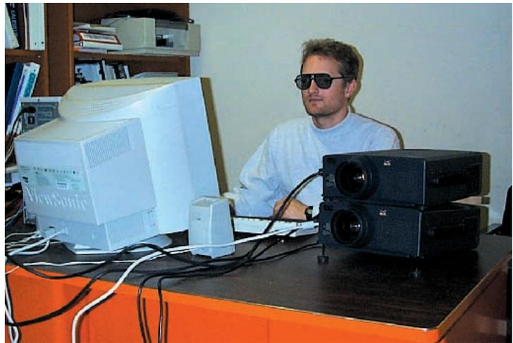
**Figure 1.** A picture showing one of the authors (Samuel T. Jones) wearing the inexpensive polarized glasses and using the visualization system. To the right are the two LCD projectors (with polarized filters) used for the right and left stereoscopic images.
